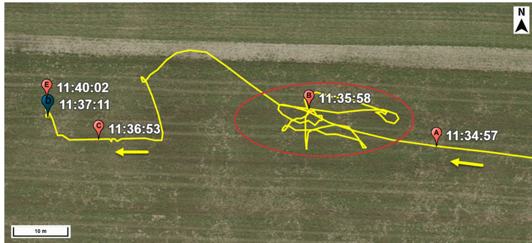
Figure 1 : Last part of the flight path before the accident. Area B (red circle) between A and C corresponds to the point where hovering exercises were carried out for about two minutes. D corresponds to the touchdown point and E to the final position of the helicopter. Source of the base map: Swisstopo, edited by the STSB.
