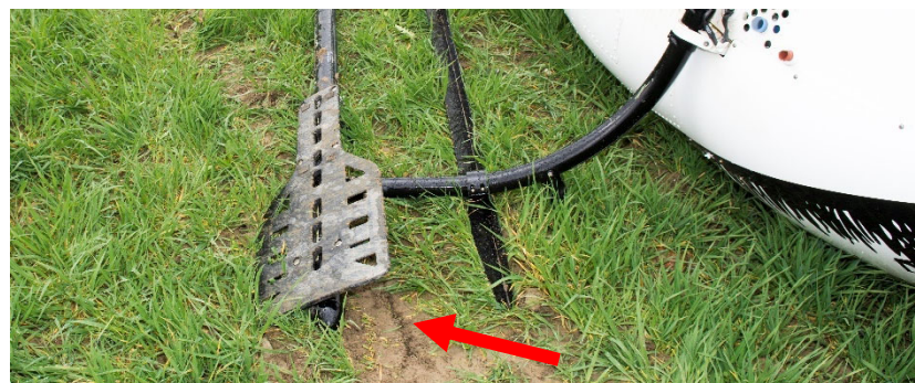
Figure 4 : Right skid with bear paw turned markedly inwards. A ground scar caused by the bear paw pressed laterally into the ground can be seen in the ground (red arrow).
